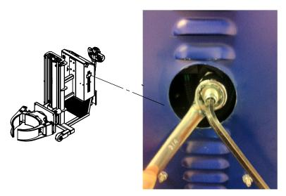
Note: Wrench shown outside the cabinet for clarity. Your machine may require removal of the back panel to loosen the jam nut and adjust pressure.
