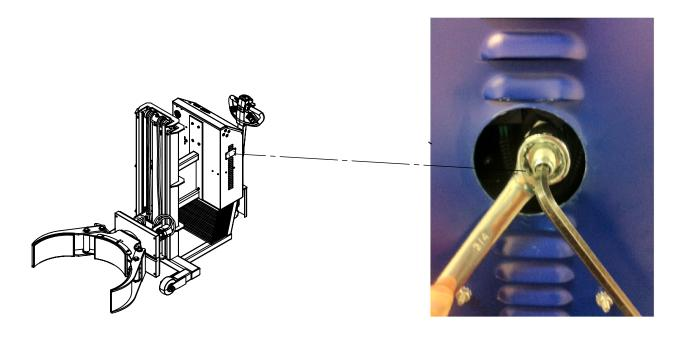
Note: Wrench shown outside the cabinet for clarity. Your machine may require removal of the back panel to loosen the jam nut and adjust pressure.
