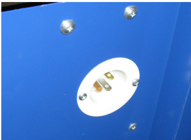
Figure 5 - Built-in 110VAC receptacle for charging.
