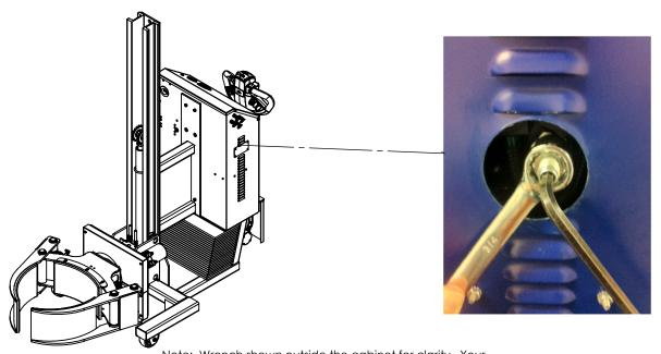
Note: Wrench shown outside the cabinet for clarity. Your machine may require removal of the back panel to loosen the jam nut and adjust pressure.
