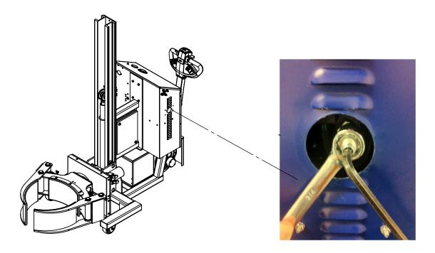
Note: Wrench shown outside the cabinet for clarity. Your machine may require removal of the back panel to loosen the jam nut and adjust pressure.
