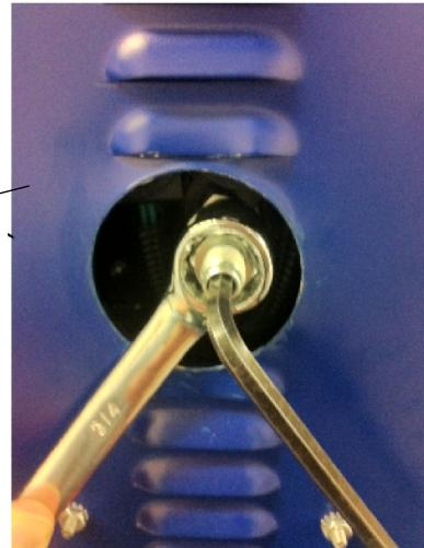
Note: Wrench shown outside the cabinet for clarity. Your machine may require removal of the back panel to loosen the jam nut and adjust pressure.
