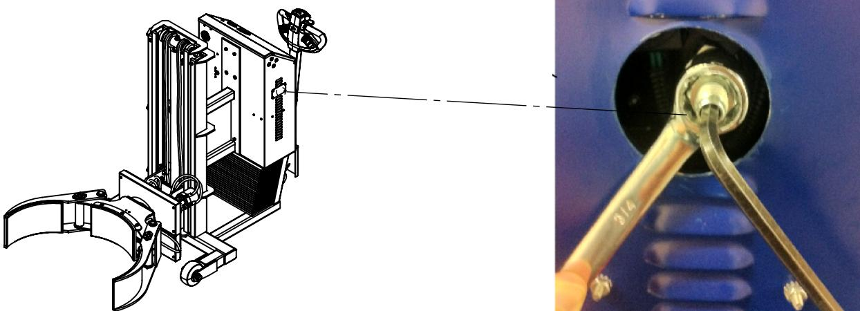
**Note:** Wrench shown outside the cabinet for clarity. Your machine may require removal of the back panel to loosen the jam nut and adjust pressure.
