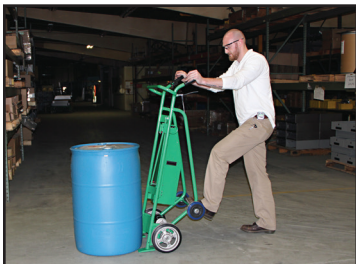
Step 2: Place shoes of truck securely against the base of the drum.
