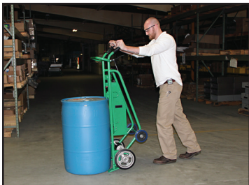
Step 3: Tip frame against the drum to engage the chime hook.
